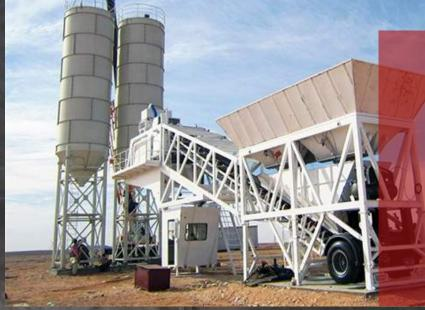
The Mobile Concrete Batching Plant is a mobile concrete production equipment that can be built and put into production on job site. Meanwhile, it is the best choice for produce ready-mixed concrete in short-term projects.
