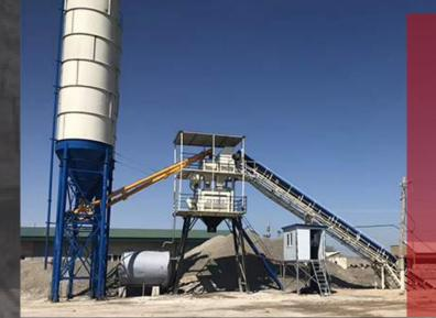
The Temporary Concrete Batching Plant usually produces concrete for specific projects. Compared with Permanent Batching Plant, the Temporary Concrete Plant adopts simple design and compact structure, reducing the initial investment cost and putting into production quickly.
