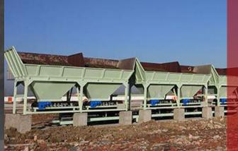
The continuous mixing plant is equipped with a continuous mixer and a continuous batching machine. It discharges materials continuously in production. At the same time, it is commonly used to produce a variety of roadbed materials, such as lime soil, cement stabilized soil, cement stabilized macadam, roller compacted concrete, etc.
