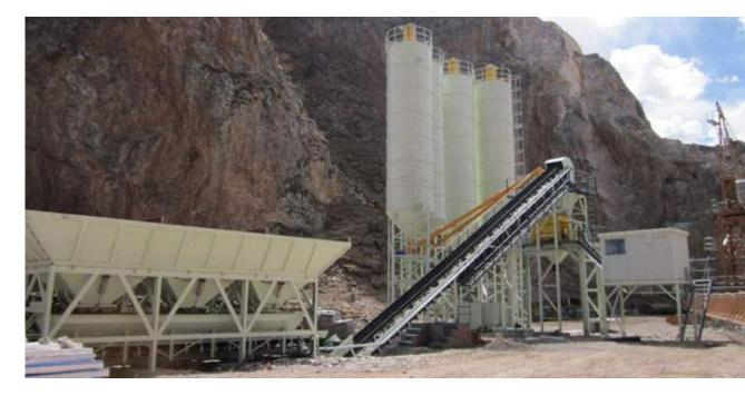
Stationary Concrete Batching Plant
