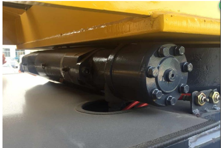
The stirring motor is too small, only use for 2.5cbm machine
